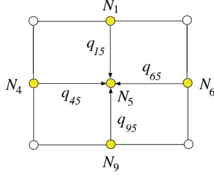
Figure 10. Five-point finite-difference scheme.
