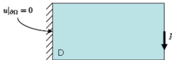
Figure 7. Definition of the minimum compliance problem for a short cantilever beam.
