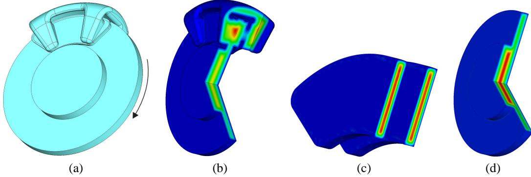
Figure 10: (a) A truck brake assembly. Approximate distance fields to the boundaries of (b) brake assembly, (c) brake pads, and (d) the disk.
