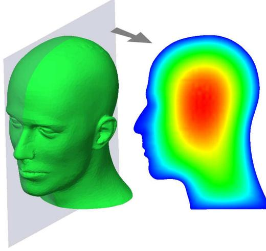
Figure 2: Distribution of the function  $u$  that satisfies homogeneous Dirichlet boundary condition (1) on the zero set of the approximate distance field shown in Figure 3(b) and approximates solution of Poisson equation (6).
