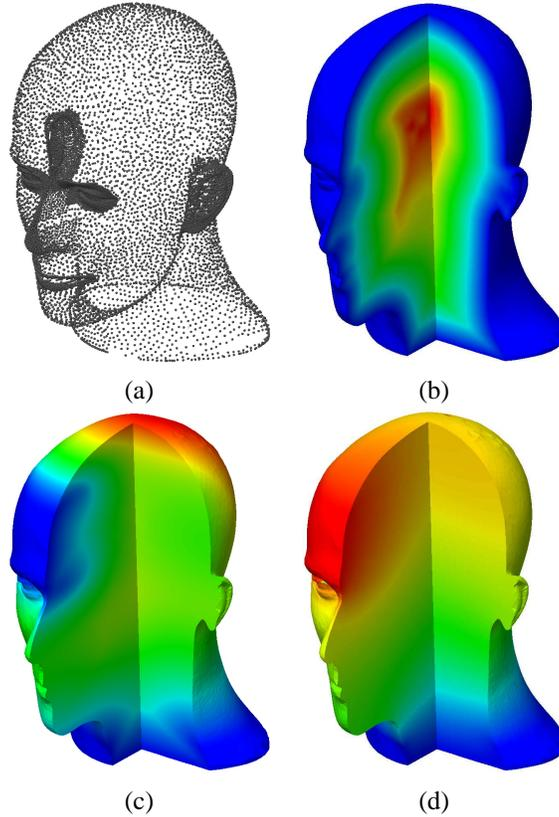
Figure 3: Modeling of temperature field in mannequin head: (a) scattered points on the surface of the head generated by 3D scanner; (b) constructed approximate distance field; (c) an approximate distance field to portions of the boundary where the value of temperature is prescribed; (d) distribution of temperature that satisfies the boundary conditions exactly.
