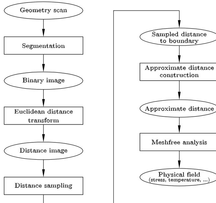
Figure 8: This figure shows the typical scheme for the “scan and solve” type of stress analysis.
