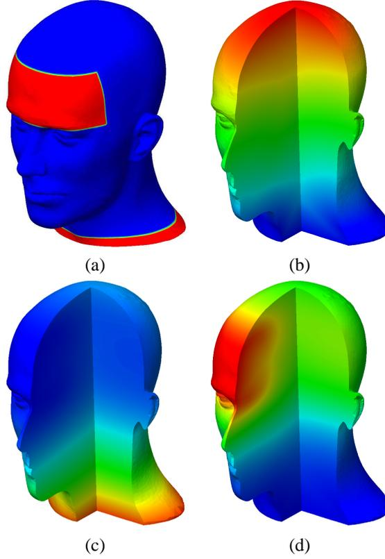
Figure 5: (a) Red colored zones depict the portions of the surface of the head where the values of temperature are specified; (b) hue values correspond to approximate distance to the lower part of the neck; (c) hue values correspond to approximate distance to the forehead; (d) distribution of function, (20), that interpolates temperature values of  $35^{\circ}C$  and  $40^{\circ}C$  prescribed on the neck and forehead respectively.
