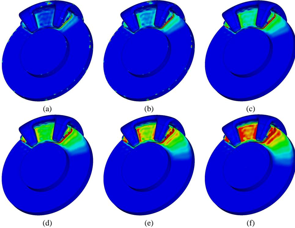
Figure 11: Distributions of transient temperature field in the truck brake assembly computed at first six time steps
