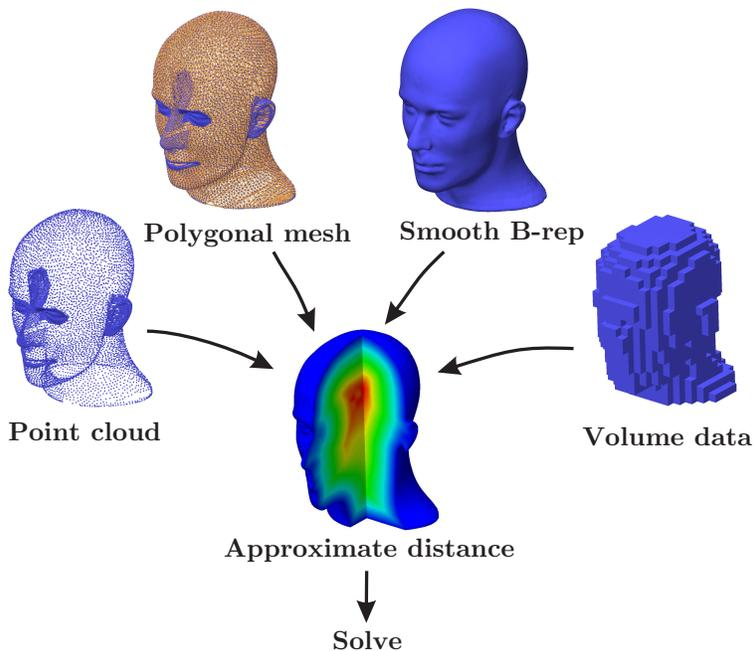
Figure 1: Figure depicts field modeling using approximate distance fields from surface points, polygonal surfaces, smooth B-rep, and volumetric data. The simplicity of the approach is in stark contrast to the multiple representation conversions required in traditional mesh-based analysis.
