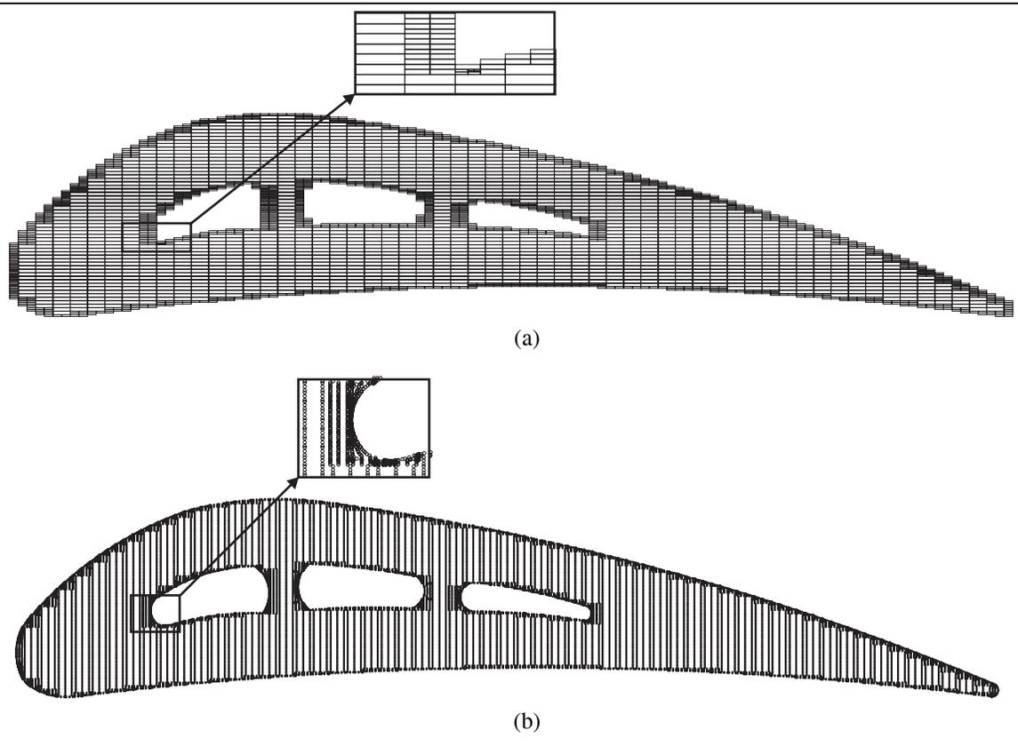
Figure 16: Adaptive integration employs hierarchical space decomposition of the geometric model
