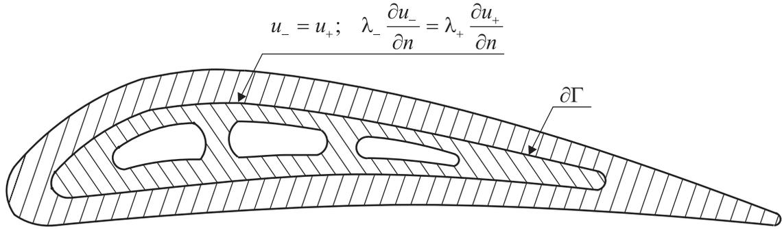
Figure 18: Boundary conditions of an ideal thermal contact are prescribed on the material interface
