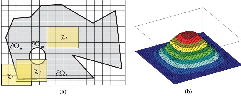
Figure 14: (a) Compactly supported basis functions satisfy only those boundary conditions that are prescribed on the boundary pieces contained in the support. (b) B-spline basis function
