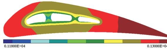
Figure 19: Temperature field in turbine blade
