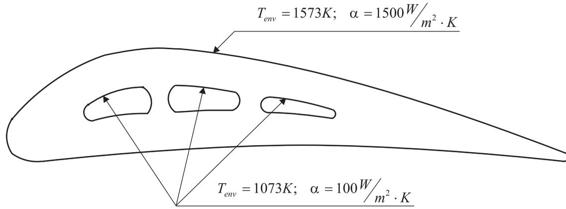
Figure 15: Boundary conditions on the outer surface of the turbine blade and on the surface of the cooling channels
