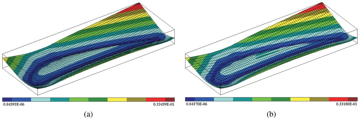
Figure 2: Distance fields to the contour of the airfoil shown in Figure 1: (a) normalized to the first order and (b) normalized to the second order
