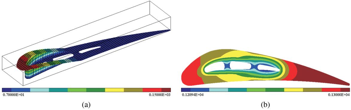
Figure 20: (a) Distribution of the thermal conductivity with discontinuities along the interface boundary; and (b) temperature field computed for heterogeneous heat conductivity presented in Figure 20(a)
