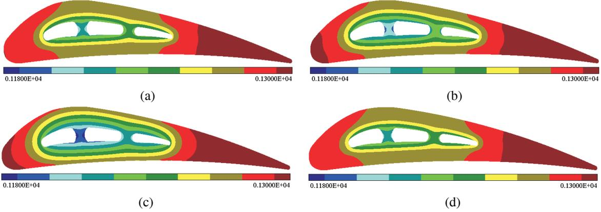
Figure 17: Temperature distributions computed for variations of the thermal conductivity presented in Figure 12
