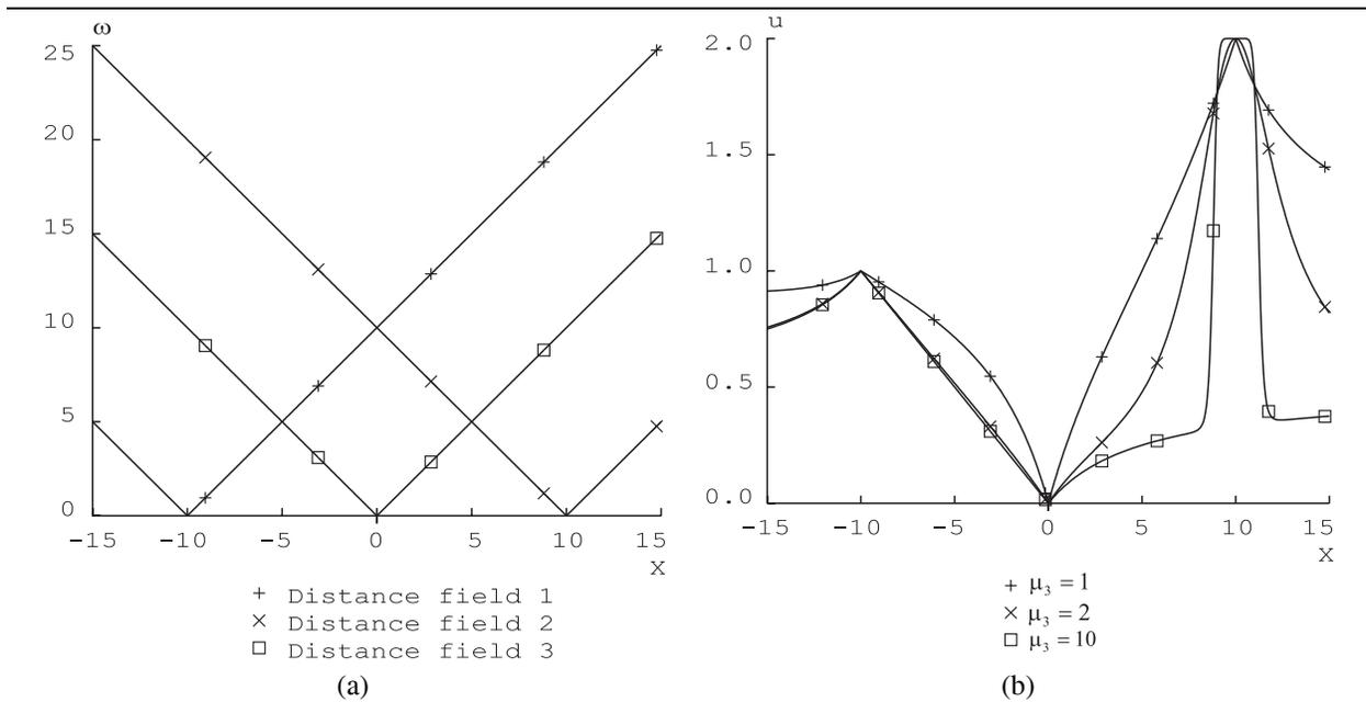
Figure 6: (a) Distance fields used for interpolation of values prescribed at points  $x_1 = -10, x_2 = 0$  and  $x_3 = 10$ . (b) Plots of the functions interpolating the values  $u_1 = 1, u_2 = 0$  and  $u_3 = 2$  prescribed at points  $x_1 = -10, x_2 = 0$  and  $x_3 = 10$  for  $\mu_3 = 1, 2, 10$
