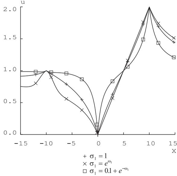
Figure 8: Plots of the functions interpolating the values  $u_1 = 1$ ,  $u_2 = 0$  and  $u_3 = 2$  prescribed at points  $x_1 = -10$ ,  $x_2 = 0$  and  $x_3 = 10$  for  $\sigma_1 = 1$ ;  $\sigma_1 = e^{\omega_1}$ ; and  $\sigma_1 = 0.1 + e^{-\omega_1}$
