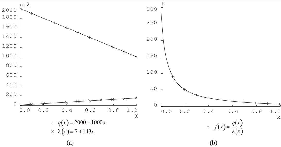
Figure 13: (a) Linear distributions of heat flux and thermal conductivity result in (b) a hyperbolic function as the boundary condition for the first normal derivative of temperature
