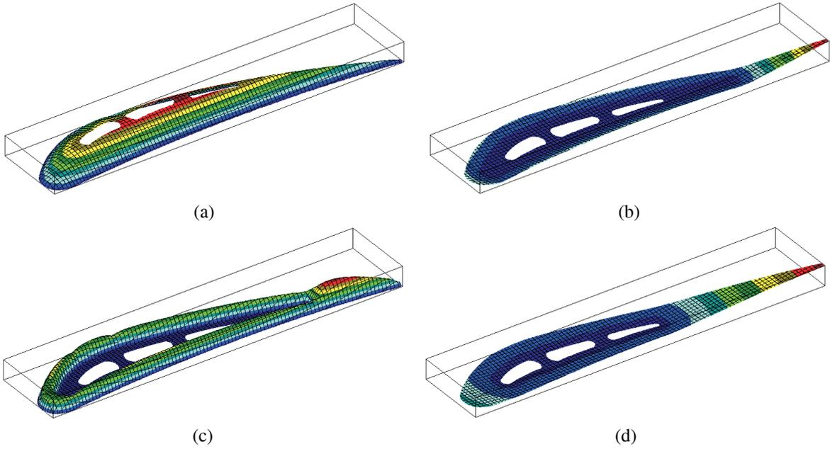
Figure 11: Approximate distance functions (a) to outer surface of the blade; (b) to the insert; (c) to outer surface of the blade and to the insert; (d) to the cooling channels
