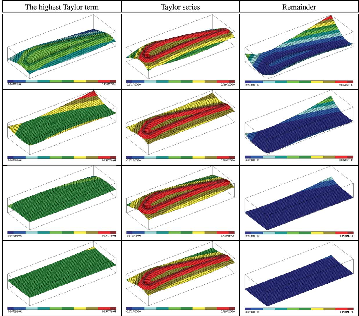
Table 1: Figures show decay of the remainder term in the Taylor series approximating the function  $e^{-50\omega}$  with an increasing number of terms. The first column shows distributions of the highest term in the Taylor series (13):  $-50\omega$ ,  $1250\omega^2$ ,  $-\frac{62500}{3}\omega^3$ ,  $\frac{781250}{3}\omega^4$ . The second column presents partial sums of the Taylor series (13), and the third column shows distributions of the absolute value of the remainder term
