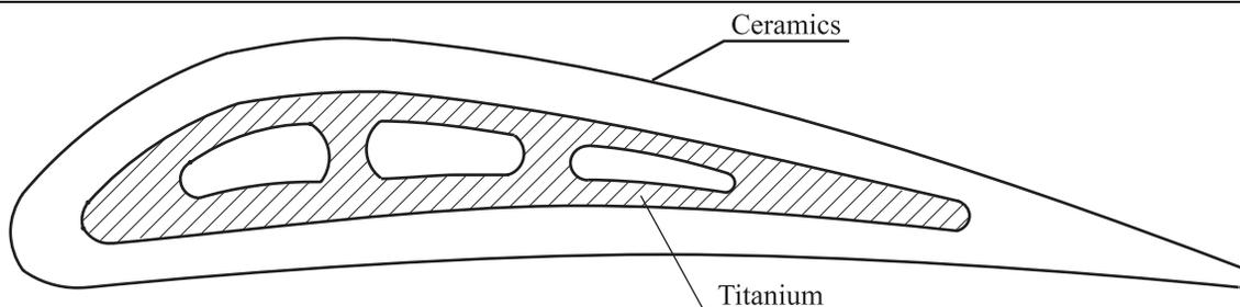
Figure 10: Cross section of a turbine blade: titanium insert surrounded by ceramics
