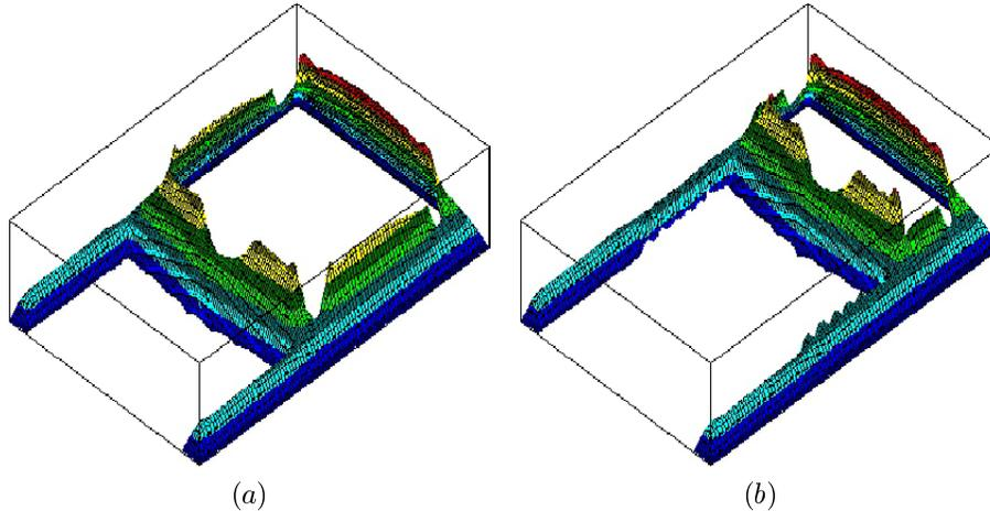
Figure 9: Temperature distributions in a engine combustion chamber
