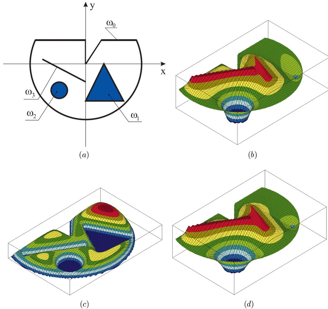
Figure 10: (a) Domain with functional values prescribed on heterogeneous loci  $\omega_i$ ; (b) function that interpolates the values prescribed on the loci; (c) function that vanishes on the indicated loci; (d) solution of boundary value problem for Laplace equation with prescribed boundary conditions
