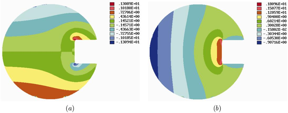
Figure 3: Stresses  $\tau_{xz}$  (a) and  $\tau_{yz}$  (b) predicted by RFM with structure (2)
